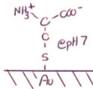
**Figure 1.** Sketch of cysteine binding to the gold surface of the electrode.
