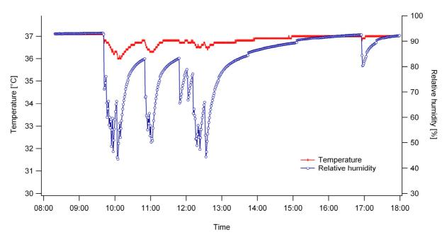
The above graph shows the temperature and humidity inside a  $CO_2$  incubator over a 10 hour day, during and after briefly opening the door. The graph shows only minor differences in temperature over the day, i.e., between 36°C and 37°C. However, it shows significant differences in relative humidity over the day, i.e., between less than 50 % and the steady state of 93 %. An important fact to note is that this incubator had not been opened all afternoon, except briefly just before 5 o'clock.
