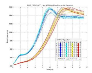
A graph is also generated showing the average values obtained from each group of 16 wells with error bars representing plus and minus one standard deviation.
